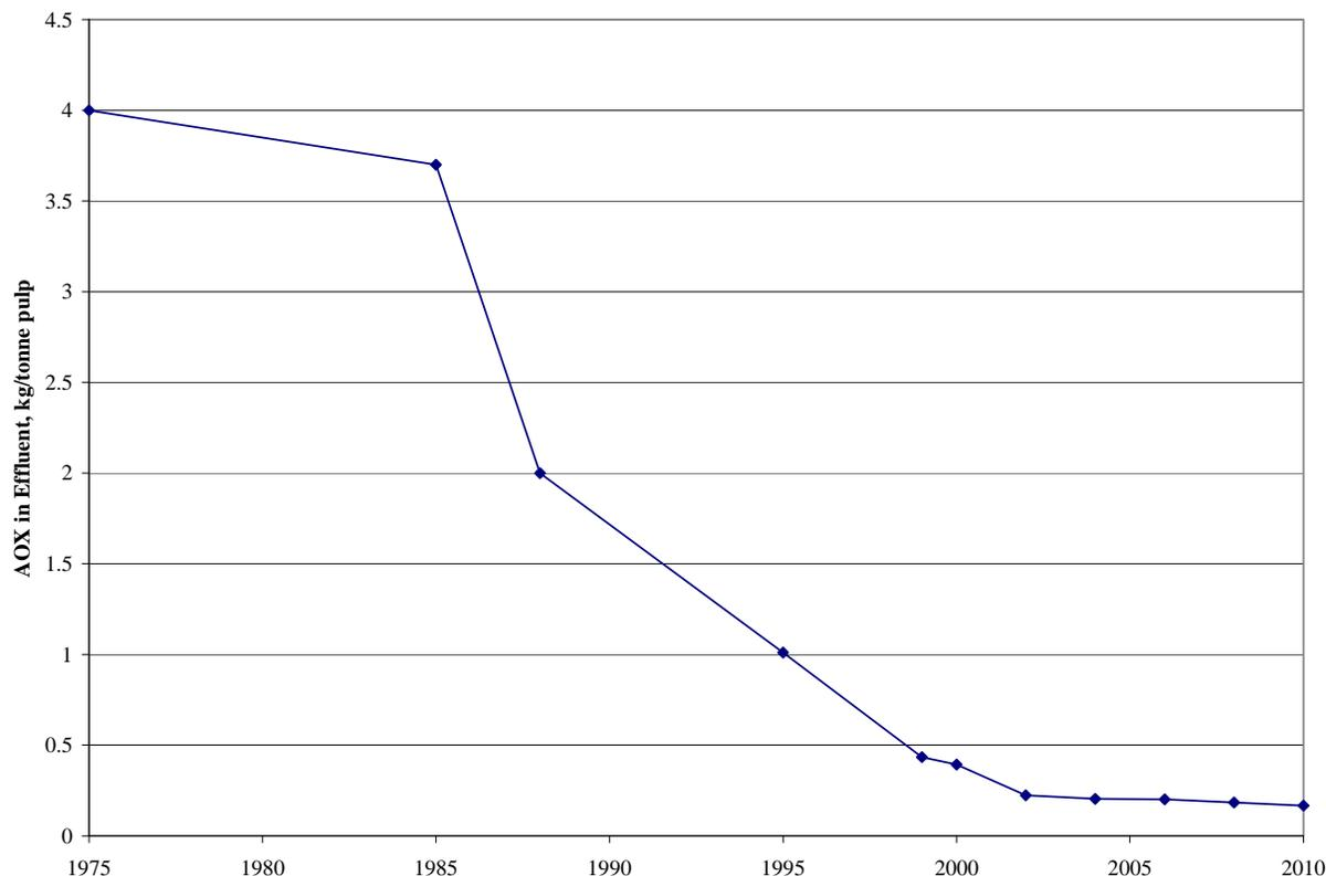
**Figure C1. Reduction in Adsorbable Organic Halides (AOX) over Time**
