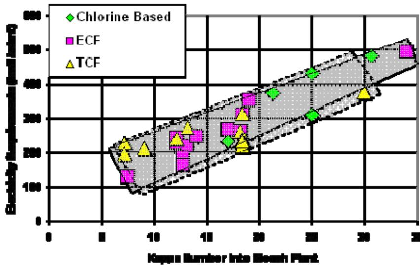
Figure C9. Electrical Energy Requirements for Bleaching Sequences When Only Considering Electricity Required for Chemical Production and Lower Electricity Values for  $O_3$  and  $H_2O_2$
