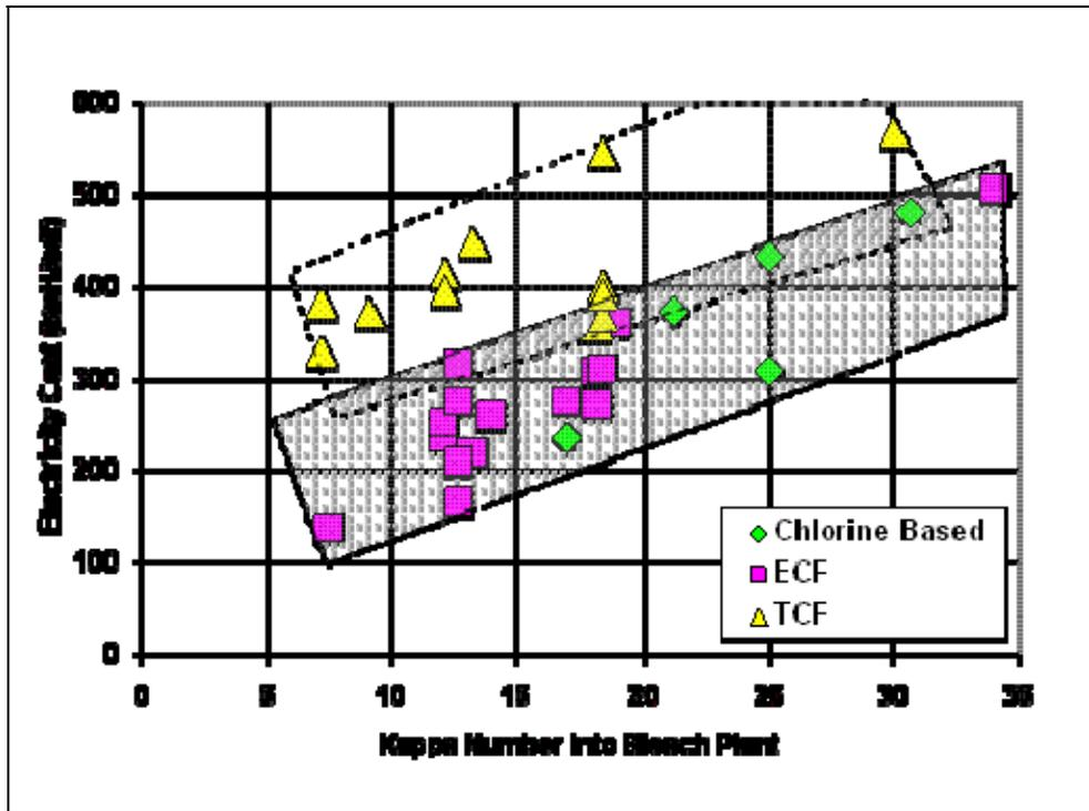
Figure C11. Electrical Energy Requirements for Bleaching Sequences When Only Considering Electricity Required for Chemical Production and Higher Electricity Values for  $O_3$  and  $H_2O_2$
