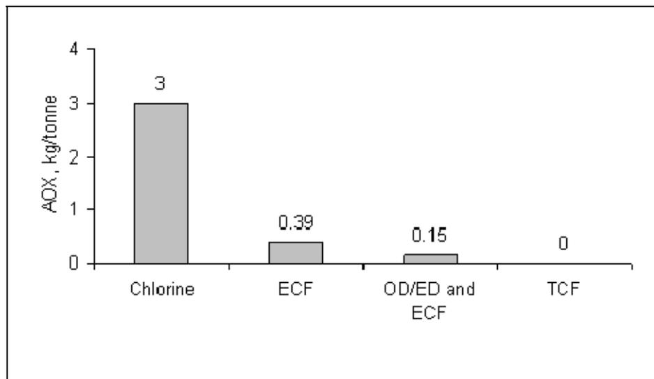
**Figure C20. AOX Loads in Treated Effluents from Softwood Bleaching Sequences**
