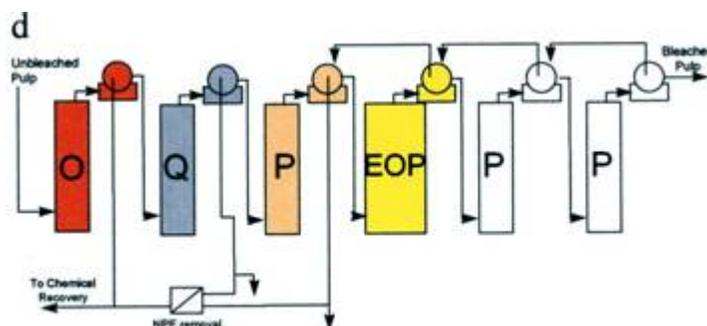
**Figure C8. Typical Totally Chlorine Free Bleaching Sequence**
