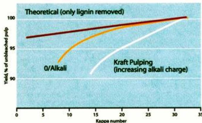
**Figure C13. Yield Loss Related to Kappa Number for Different Delignification Approaches**
